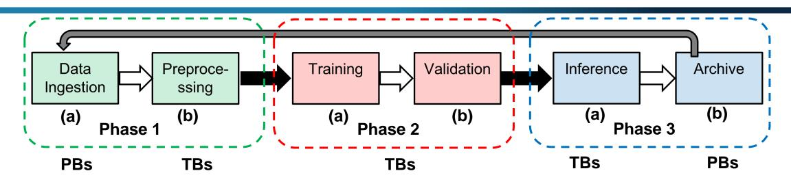
(a) Ingest massive *objects* via bulk-insert (streams) across data-sources/clouds/data-centers, etc.
